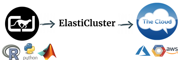
Fig. 2. ElastiCluster-ClusterJob stack first provisions a personal cluster in the cloud using ElastiCluster, and then links ClusterJob to this cluster to run ambitious experiments involving many parallel jobs. Experiments are documented reproducibly, and can be retrieved at a later time via ClusterJob interface. This stack is agnostic to the choice of cloud provider and programming language.
